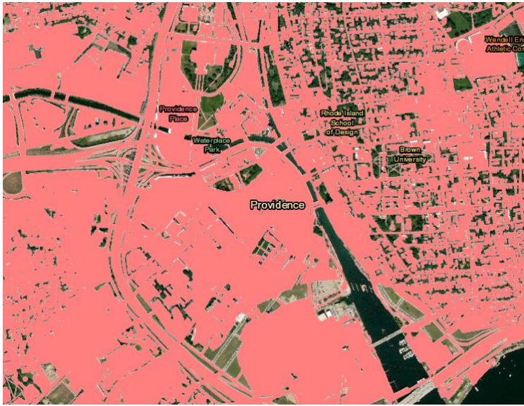
Figure 18: Impervious Surfaces in the centers of Providence and Newport. Impervious surfaces on these maps of Providence and Newport are highlighted in red. Source: From RI GIS, data from 2003-2004 and 2011. Available at https://www.arcgis.com/home/webmap/viewer.html?webmap=a5d0ee6edbf4dd3962579c9def9dd2e
